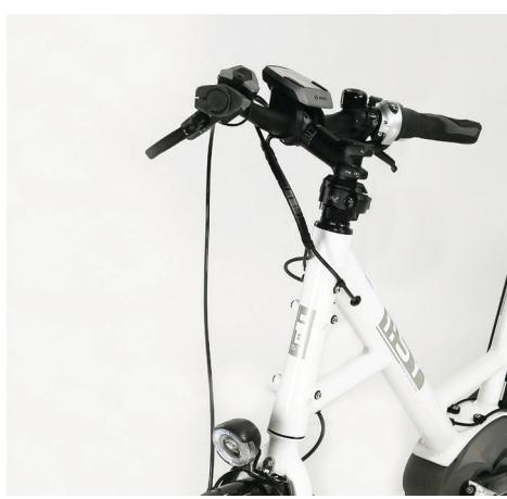
**LEFT** The I:SY only reveals its true size once you've used the tool-free Speedlifter stem to turn the bars through 90 degrees, and folded the folding pedals. This makes this pedelec into a very thin, low package, so that it can be easily stowed away, for example in a mobile home or car. This ability could also be just as much of an advantage in a cramped garage, or when taking it with you on public transport.
