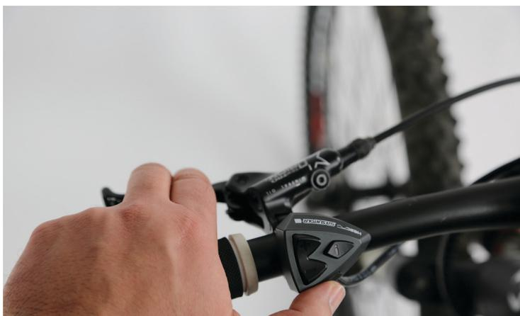
**LEFT** The small operating console on the handlebars and the elevated display on the stem look a little out of place on this pedelec. One practical touch is the Micro USB charging port which can be used to provide power to additional digital devices on the handlebars. The hydraulic Tektro Orion disk brakes are easy to modulate using the two-finger brake levers. The Rockshox suspension fork and Shimano XT shifter units both represent state of the art technology.
