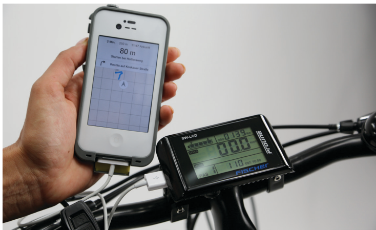
LEFT A very practical detail: the display has a USB port which can be used without adaptors for any standard USB charging cable.
