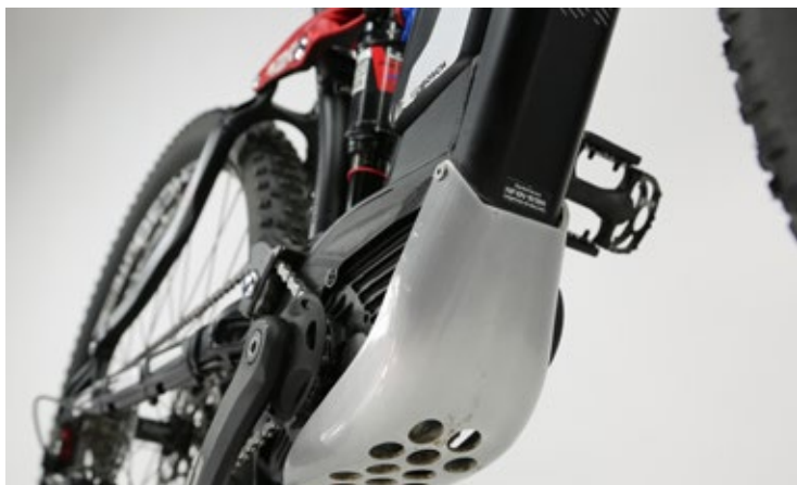
LEFT The mid motor is elegantly and robustly integrated on this Bulls off-road pedelec, and it is far nicer than the original Bosch plastic housing, which in contrast looks cheap. The massive aluminium impact guard gives credible protection to the drive against grounding. It is just a little tedious getting mud out of the holes after riding through it.
