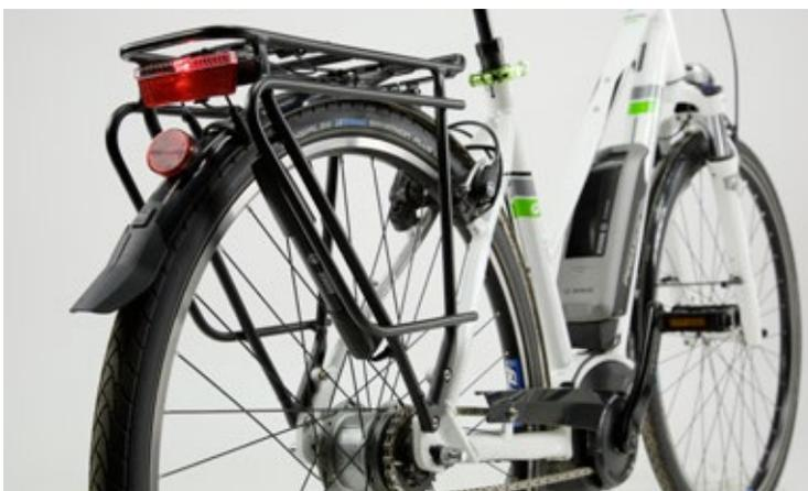
**LEFT** The Premio E8 is thoroughly equipped for touring, and with the electric drive system placed well forwards you can add more weight onto the rear carrier before the bike becomes back-heavy. The solid rear stand also provides good stability when you are loading up with panniers. Also very practical for touring: threaded bosses for mounting a drinks bottle cage are provided ready to use on the top tube.
