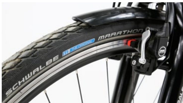
LEFT The strengths of the Raleigh Dover XXL show in the details. Note here the extra strength from the hollow-section rims, the red Magura brake blocks chosen for maximum braking power, and the well-proven Schwalbe Marathon tyres. Even if you don't load up with the full permitted 142.7 kg payload, with the Dover XXL you at least have the reassurance that you're not running close to the limits of the materials.
