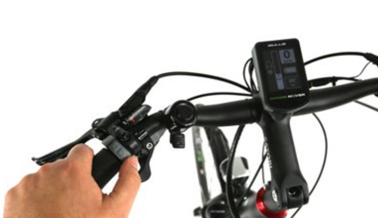
**LEFT** Rather like the cockpit of a modern car, the *Greenmover's* handlebars are crammed with user controls, so it takes a while to work out what is what. But after a short familiarisation you quickly learn to appreciate the wide-ranging functionality. Unfortunately the push assist is not located on the lower media button shown on the picture: this would be ergonomically perfect when pushing the bike.
