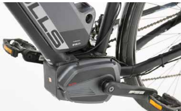
LEFT The battery pack, placed perfectly for centre of gravity, has a stupendous 615 Watt hours capacity, and the whisper-quiet Brose mid motor, which operates smoothly but with real power when required, are a fantastic pairing. What makes the Brose motor special is that it is not bolted onto the frame, but rather to optimise structural efficiency and weight it is fitted from the side into a sort of oversized bottom bracket shell.
